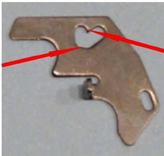
2. Here's a modified bolt stop. The cuts allow the bolt stop to depress so as to facilitate the bolt traveling over the stop and fully forward.
